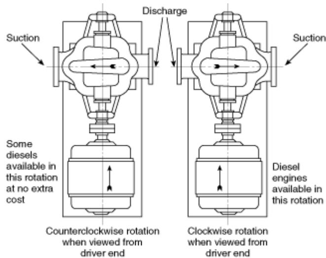
(c) *Vertical Pump Shaft Rotation.* The rotation of a vertical pump can be determined by looking down upon the top of the pump. [See Figure A-2-17(c).] If the point of the shaft directly opposite revolves from left to right, the rotation is right-handed [or clockwise (CW)]. If the point of the shaft directly opposite revolves from right to left, the rotation is left-handed [or counterclockwise (CCW)].
