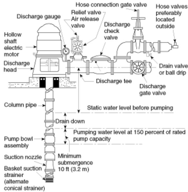
**Figure A-4-2.2.2 Vertical shaft turbine-type pump installation in a wet pit.**
