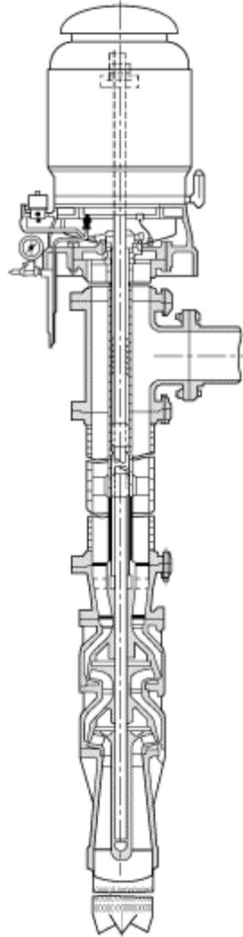
**Figure A-4-2.2.1 Vertical shaft turbine-type pump installation in a well.**
