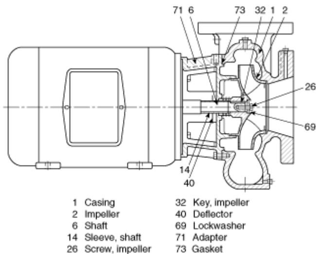
**Figure A-3-1.1(b) Overhung impeller — separately coupled single stage — frame mounted.**
