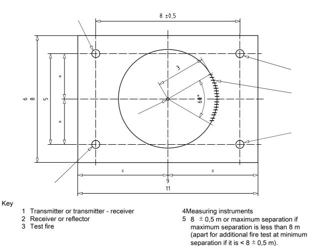
Figure B.1 -Plan view of detectors, position of fire and measuring instruments
