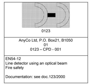
Figure ZA.1 - Example of CE marking
